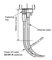
· Do not forcefully bundle or twist the cables in the bent portion (sliding portion) during installation. Avoid bundling the cables in or near the movable portion. Instead, bundle the cables at least 100mm away from the movable portion.
