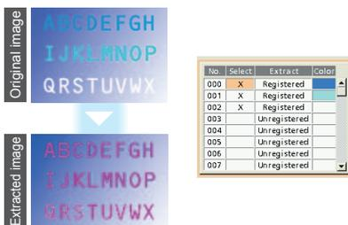
Capable of reliably reading deformed, distorted or partly chipped characters
