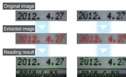
2D code reading: Codes with contrast fluctuations, out-of-focus codes, and codes with hidden or chipped portions can also be read.
