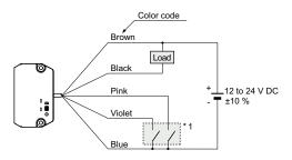
Non-voltage contact or NPN open-collector transistor
