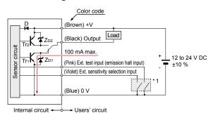
Symbols ... D: Reverse supply polarity protection diode ZD1, ZD2: Surge absorption zener diode Tr1: NPN output transistor Tr2: PNP output transistor
