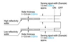
From the above, for determining the position of the wafer from the sensing signal, calculate the center position of the signal's ON region, while taking into consideration the response time.
