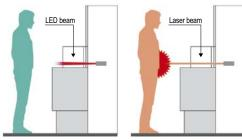
LED beam mapping sensor Laser beam mapping sensor
