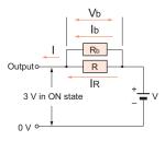
Provided that bleeder resistance is "Rb", electric current flowing to "Rb" is "lb", voltage within Rb is "Vb", electric current flowing to R is "IR", load current to the sensor is "I", and supply voltage is "V";
