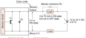
In the case that load current is under 3 mA when the output is in the ON state
