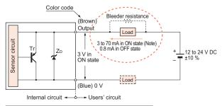
Symbols ... ZD: Surge absorption zener diode Tr: PNP output transistor
