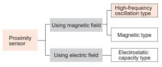
Panasonic Industrial Devices SUNX proximity sensors are high-frequency oscillation type inductive proximity sensors.
