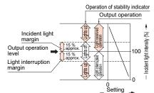
In case of the NA2-N series, NA1-PK5 series, NA1-5 series and NA1-PK3 series, this is the stable incident beam indicator and lights up when the incident light margin is exceeded.
