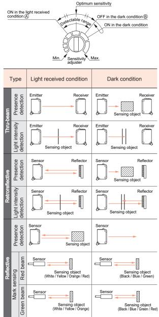
For models equipped with auto sensitivity setting function, sensitivity adjustment is performed with a single touch of a button without the sensitivity adjustment described above.
