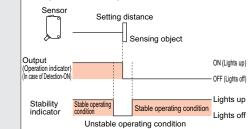
The stability indicator (green) of the EQ-30 series shows the safety margin of the incident light intensity, not that of the object distance. Hence, the distance at which it lights up / off depends on the object reflectivity and is not at all related to the output operation. Do not use the sensor when the stability indicator is off (unstable light received condition), since the sensing will be unstable.
